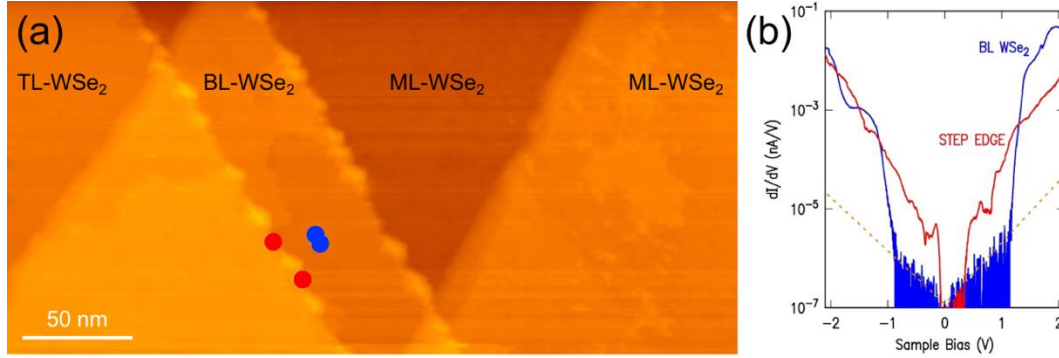
Figure 3. Topography and electronic characterization of aged WSe 2 , acquired at low temperature of 5 K. (a) STM image ( V_b = 2 V, I_t = 0.02 nA) of the oxidized WSe 2 surface showing edges between ML and BL WSe 2 and between BL and TL WSe 2 . (b) dI/dV spectra measured at the step edge and the BL WSe 2 locations indicated in (a).
